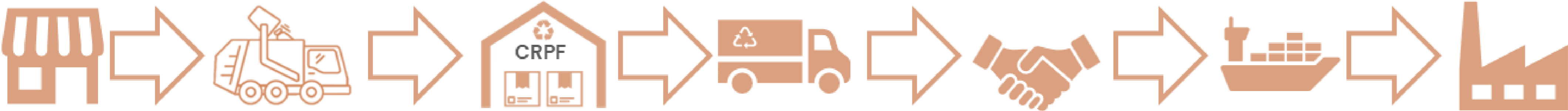
Discarded material is collected, baled at a CRPF, passed through a broker and sent to a responsible end market
